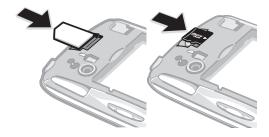
Remove the battery cover, then insert the SIM card and the memory card in the relevant slots.
