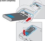
Replace the battery cover, and tighten the two screws, being careful not to overtighten.
