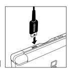
IMPORTANT: Be sure the DC Connector Plug is facing in the correct direction before inserting into the connector to avoid damaging either the plug or connector.
