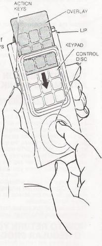
To operate the directional disc, press your finger on the outer edge and slide your finger around the edge to change direction of object you are moving. You have the ability to move
