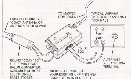
NOTE: FOLLOW THE DIRECTIONS IN YOUR TV OWNERS MANUAL OR ON THE BACK OF YOUR SET FOR CHOOSING BETWEEN THE ALTERNATE "COAX" VHE TERMINAL AND THE FLAT "TWIN LEAD" VHF SCREW TERMINALS. YOU MUST SELECT THE FLAT "TWIN LEAD" VHF SCREW TERMINALS WHEN USING THE SWITCH BOX.
