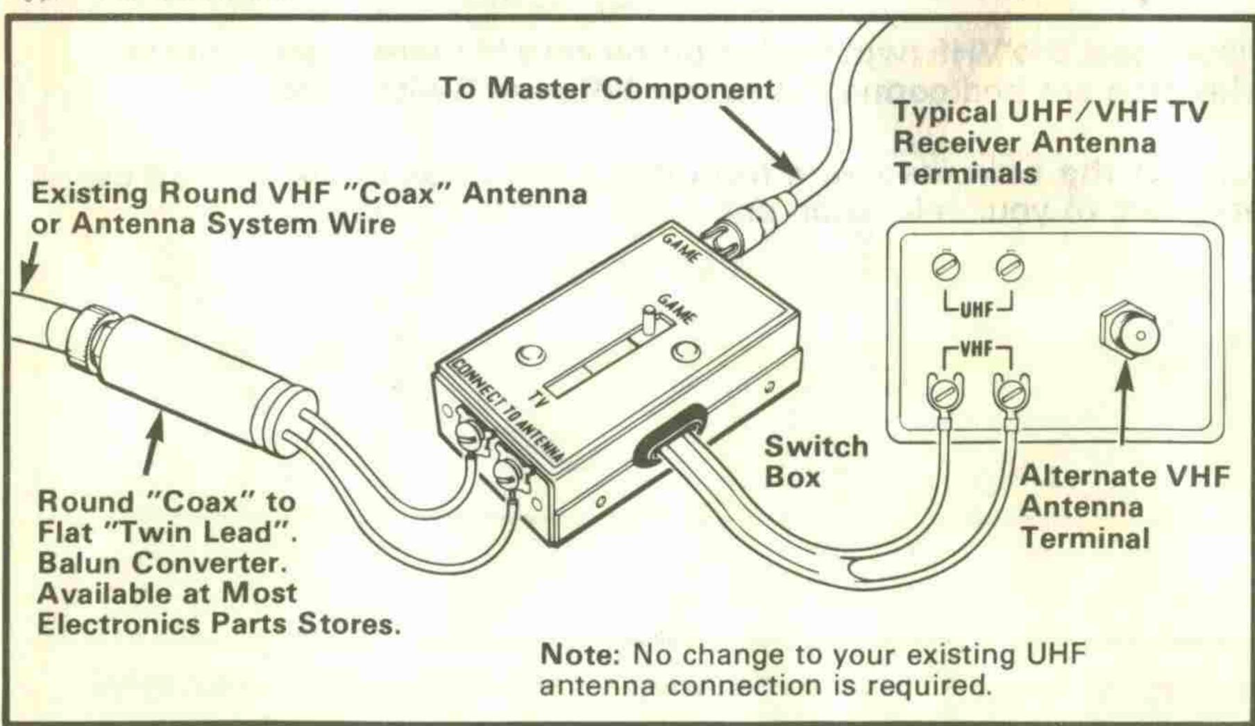
Note: Follow the directions in your TV Owners Manual or on the back of your set for choosing between the alternate "Coax" VHF terminal and the flat "Twin Lead" VHF screw terminals. You must select the flat "Twin Lead" VHF screw terminals when using the Intellivision switch box.
