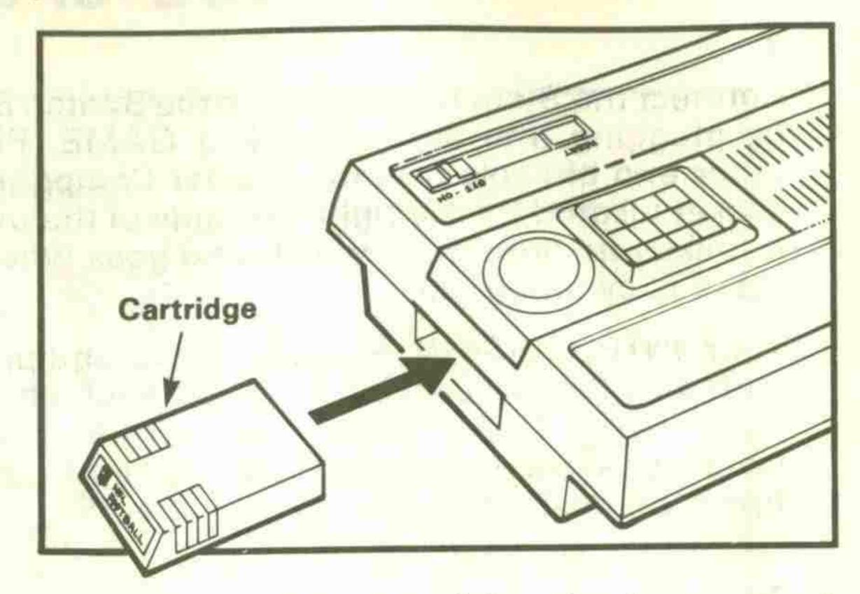
To remove the cartridge, simply pull it straight out of the slot. However, the Master Component should be turned to OFF when the System is not in use.
