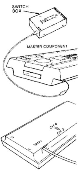
1. Connect the Switch Box cable to the Switch Box by plugging it into socket marked GAME CORD. Plug other end of cable into the Master Component socket in the rear of the Master Component on the right hand side. It makes no difference which end goes where; cable is symmetrical.
