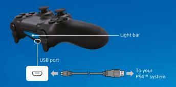
To charge your controller when in standby mode, you must first checkmark the [Supply Power from USB Ports] option in (Settings) > [Power Saving Settings] > [Set Functions Available in Standby Mode].
