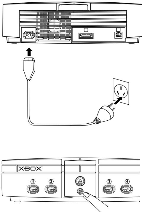
Plug the power cable into the Xbox console, and then fully insert the plug into the power outlet. See General Electrical Precautions on page 5 for more information.
